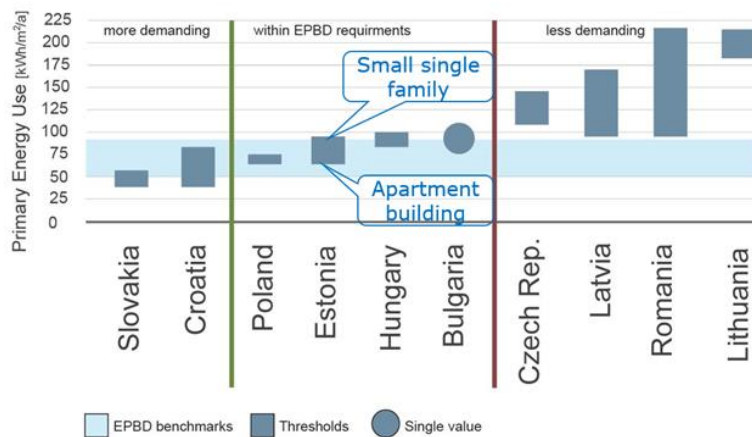
Figure 2. A comparison of NZEB requirements between Estonia and other Eastern European countries.
